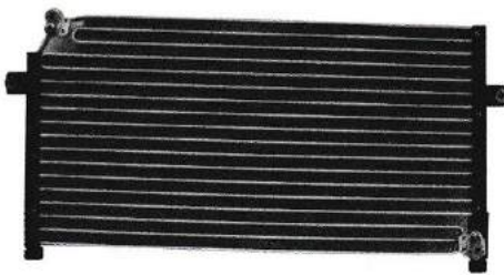
CAR MODEL: NISSAN BLUEBIRD-U12 MODEL: 日产蓝鸟 U12( 日产千里马 J30 ) YEAR: 89-91 SIZE: 730×362×22
